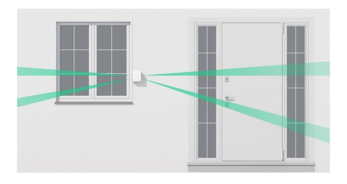
If one side of the detector is used to protect a door, and the other to protect a window, the detector is installed at the height of **0.5 to 0.6 meters from the window sill**. If the detector is placed close to a window, the Near area detection option should be enabled (the **Near area detection** switch on the back of the detector). The option reduces the blind spot near the detector.
