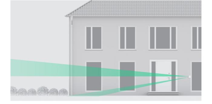
DualCurtain Outdoor includes two opposing curtain motion detectors. The detection distance is adjusted separately for each side with the **Detection Distance** scrollbars on the back of the detector.
