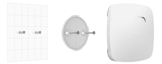
1. Fix the SmartBracket panel on the ceiling using bundled screws. If you use any other attachment tools, make sure that they do not damage or deform the attachment panel.
