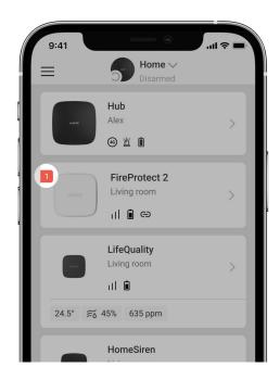
If FireProtect 2 malfunction is detected (for example, there is no connection with the hub), the malfunction counter is displayed in the
