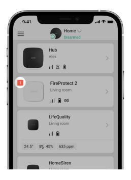
When a malfunction is detected, the Ajax app displays a malfunction counter on the device icon. All malfunctions are indicated in the device's states. Fields with malfunctions will be highlighted in red.
