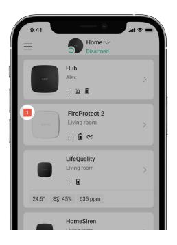
When a malfunction is detected, the Ajax app displays a malfunction counter on the device icon. All malfunctions are indicated in the device's states. Fields with malfunctions will be highlighted in red.
