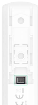
We recommend installing the wired detector at a distance no longer than 1 meter to GlassProtect. Longer wire length increases the risk of its damage and reduces the quality of communication between the detectors.
