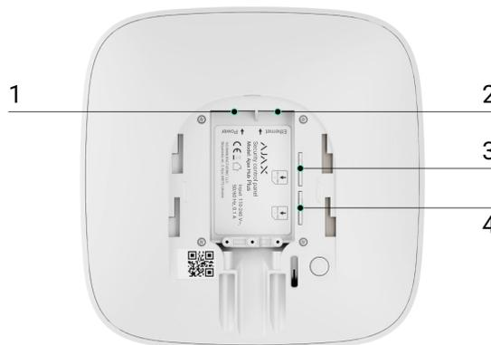
1 – Power Socket, 2 – Ethernet socket, 3, 4 – Slots for micro-SIM cards connection
