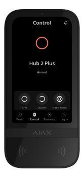
KeyPad TouchScreen can arm and disarm the entire facility or specific groups, and activate **Night Mode**. Use the **Control** tab to change the security mode. You can control the security using KeyPad TouchScreen
