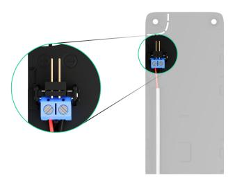
**4.** Route the cable in the cable channel. An example of how to output the cable from the bottom of the keypad:
