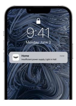
LightSwitch continuously checks its power supply parameters. If LightSwitch controls the power of a lighting device with insufficient power (up to 5 W), the system will notify the users of the Ajax system. In this case, it is necessary to replace the lighting device with a similar one with higher capacity or to connect a bundled capacitor in parallel with the lighting device.
