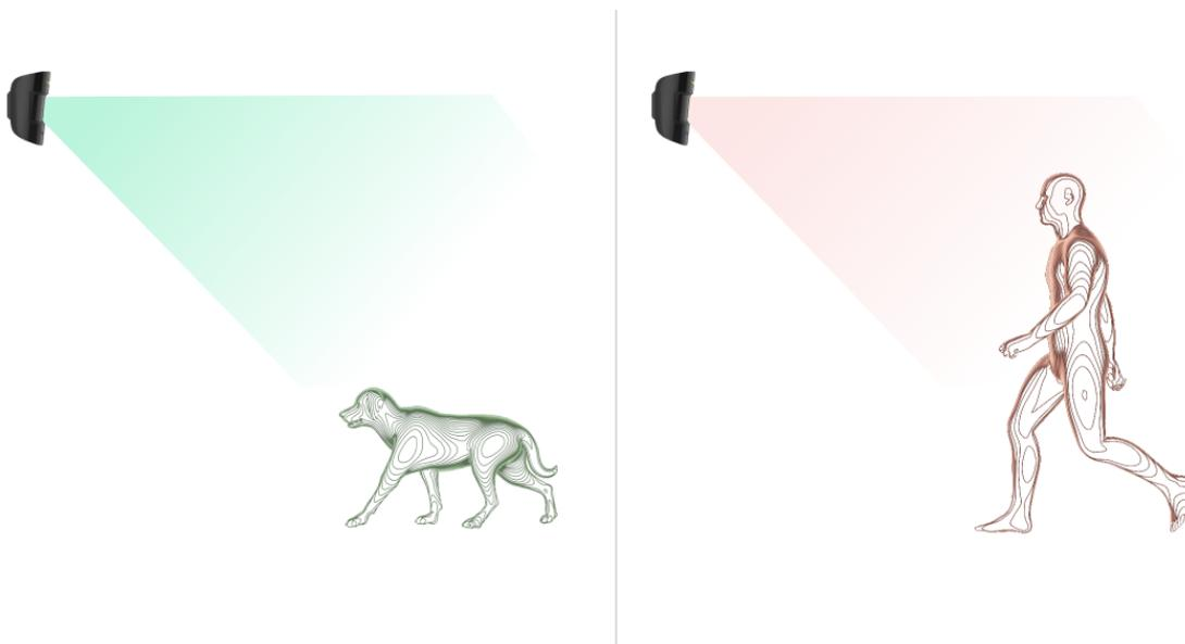
The detector is installed **at a height of 2.4 meters** without any obstruction to its view – for example, in the corner of the room, where the view won't be blocked by closets or other furniture.
