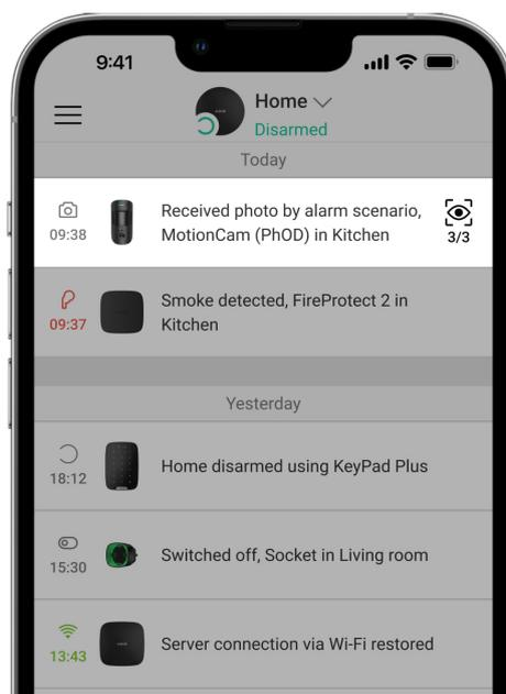
The **Photo by scenario** feature allows you to create a scenario for motion detectors with photo verification. These detectors will take pictures in case of alarms from specified Ajax devices.
