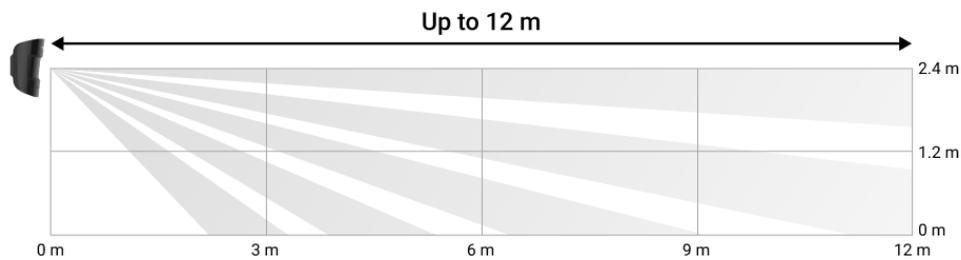
When installing the detector, perform the Detection Zone Test. This allows you to check the operation of the device and accurately determine the sector in which the detector registers motion.
