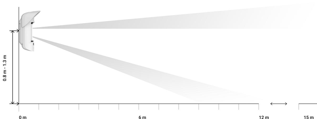
The detection distance is adjusted using the **Detection Distance** scrollbar on the rear panel of the detector. When choosing the installation location, consider the maximum detection range of the detector. It depends on the
