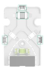
**4.** Remove the rubber sealing plugs that protect the top and side screws of the swivel mount. Do not use sharp or spike tools to prevent damaging the sealing plugs.
