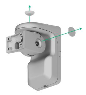
**4.** Unscrew the top screw and the holding screw at the bottom of the swivel mount. Disassemble the rear part of the swivel mount by sliding it up.
