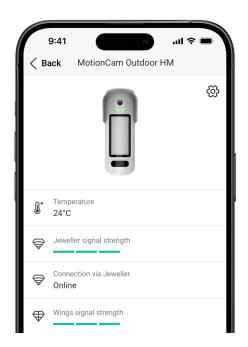
The states include information about the device and its operating parameters. The states of MotionCam Outdoor HighMount (PhOD) Jeweller can be found in Ajax apps:
