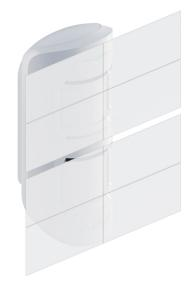
**Masking** is an attempt to block the view of the detector by painting over it, covering it, placing an obstacle in front of the detector's lens, or otherwise.
