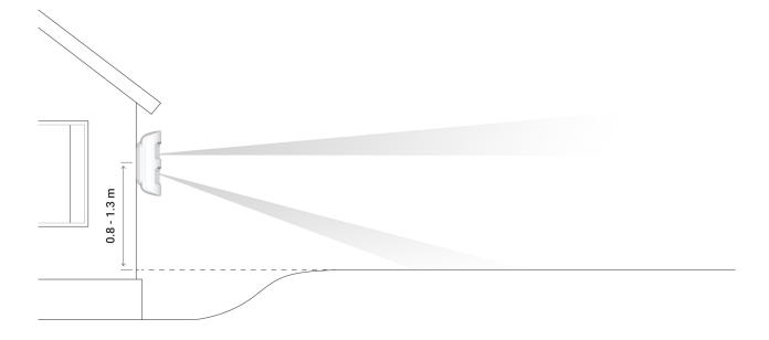
We recommend placing the detector in a corner so that it has no "blind" zones and is harder for an intruder to bypass. For example, in the corner of a fence. Furniture, plants, and ornamental and glass structures should not obstruct the view of the detector or its camera.
