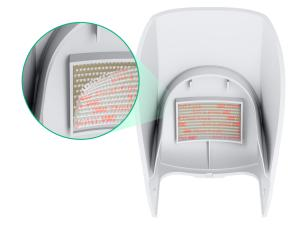
**2.** Put Hood on the MotionProtect Outdoor — part of the tape will stick to the detector's enclosure.
