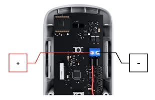
**9.** Connect the other end of the cable to the power source following the polarity. The power supply must be de-energized at the time of connection.
