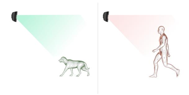
The detector must be installed at 2.4 meters without obstruction to its view. For example, in a corner where the view will not be blocked by a closet or other furniture on which a pet can climb.
