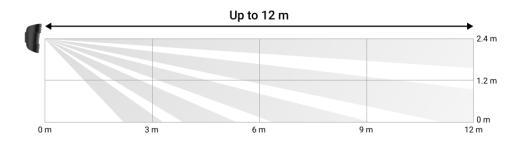
When installing the detector, perform the **Detection Zone Test**. This test is implemented to provide the possibility to check the device's operation and determine the sector in which the detector registers motion.
