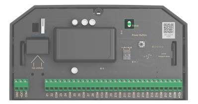
The MultiTransmitter LED indicator may light up in white, red, or green depending on the device status.
