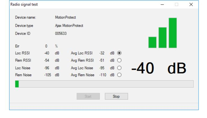
The results of the test are shown in the configuration software (Picture 7) as 3 indication bars, and by the sensor light. The test results can be the following:
