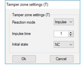
When "Bistable" mode is chosen for reaction, service zone reacts by closing/opening the output depending on "Initial state" setting (NC/NO) until the zones returns to the initial state. When the initial state is changed, green light "12" of the appropriate service zone (Picture 1) turns on.
