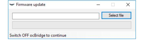
Then, it is necessary to power the receiver off with switch "10" (Picture 1) and turn the device on again. After switching on, the upgrade process begins automatically. In case the process was accomplished successfully, there is a message "Software upgrade is accomplished" and the receiver is ready for work.
