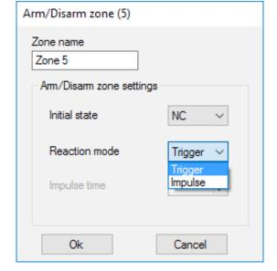
Arm/disarm zone can be set to initial state NC or NO. When the keyfob is registered, in arm/disarm zone two buttons are added simultaneously: button 1 — arming and button 3 — disarm. To arm, the zone reacts with closing/opening the output, depending on the setting "Initial state" (NC/NO). When this zone is activated, the red light corresponding to it turns on, and when it is deactivated, the light "3" (Picture 1) is off.
