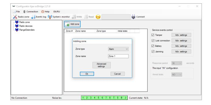
Then, appropriate "Zone type" and settings is to be selected (consult Managing the central unit of the present manual). To add a device chose necessary zone and click "Add a device" button. Then, a "Adding new device" window appears and it is necessary enter sensor's identifier (ID) applied on it below QR code, then click the "Search" button (Picture 4).
