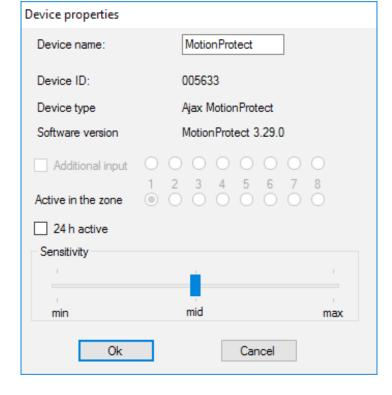
When an additional wire sensor is connected to the external digital input of the wireless sensor, in the properties activate the checkbox "Additional input" (Picture 5). If a sensor (for example, a LeaksProtect) is designed for working 24 h, activate in the checkbox properties "24 h active". 24 h sensors and normal sensors should not be placed in the same zone! If necessary, adjust the sensor's sensitivity.
