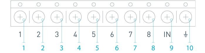
Other 5 outputs of ocBridge Plus are service zones and correspond to the service inputs of the alarm system central unit.
