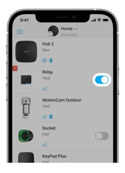
In <u>Ajax apps</u>, you can switch on and off electrical appliances connected to an electrical circuit controlled by Relay Jeweller.
