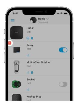
In case of Relay Jeweller fault (e.g., no Jeweller signal between the hub and the relay), the Ajax app displays a malfunction counter in the upperleft corner of the device icon.
