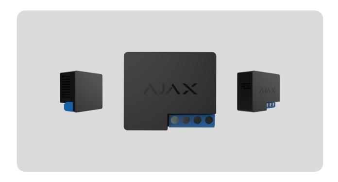
**Relay Jeweller** is a dry contact relay to control a power supply remotely. The relay's dry contacts are electrically isolated to the power supply circuit of the device. Relay can be used in both low-voltage and domestic power grids. The device features two types of protection: voltage and temperature.
